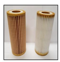
Original equipment manufacturer, Volkswagen, superseded cartridge filter 06K115466 with 06L115562B.
