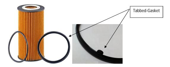
This tabbed-gasket utilized for Audi and Volkswagen applications has a concave indentation on the inside diameter. This gasket is designed in such a way specifically to reduce the effort required to install the cap into the housing. Function of the gasket is improved by this design.
