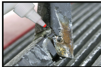
Spraying hinge to flush & lubricate
